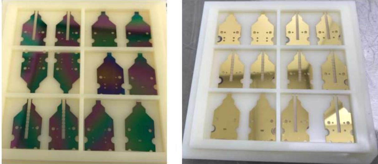
Figure 2: Fabricated chips before (left) and after (right) metallization.
